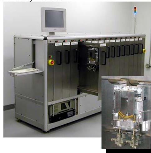
Figure 4: High performance curing system (Inset: Aerospace cable assembly in precision mechanical fixture)
