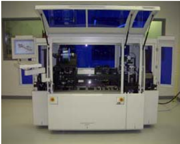
Figure 2: Automated Termination Assembly System
