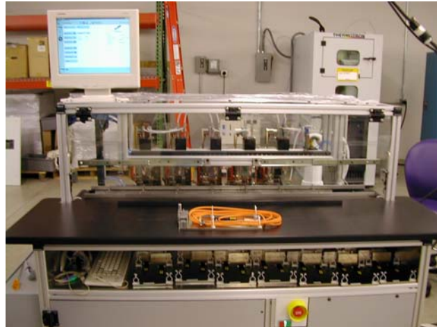
Figure 3: Automated End Face Polishing System
